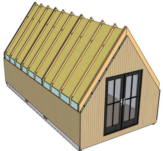
Implement door/other openings within structure and fit all required flashings
